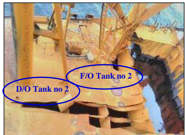
Port side F/O no 1, 2 and D/O tank plates blown off
