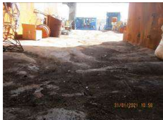
Bulged & deformed engine room casing bulkhead and upper deck
