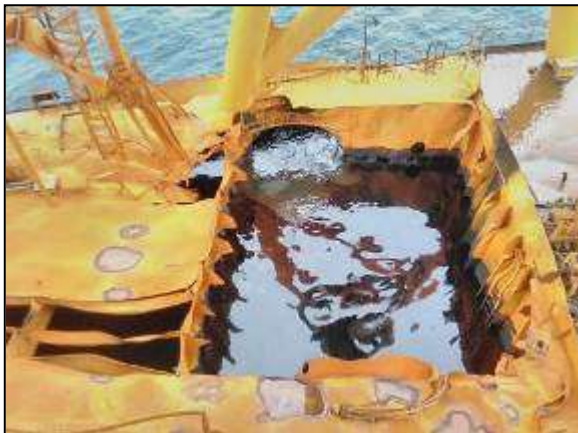
Port side F/O no 1, 2 and D/O tank plates blown off
