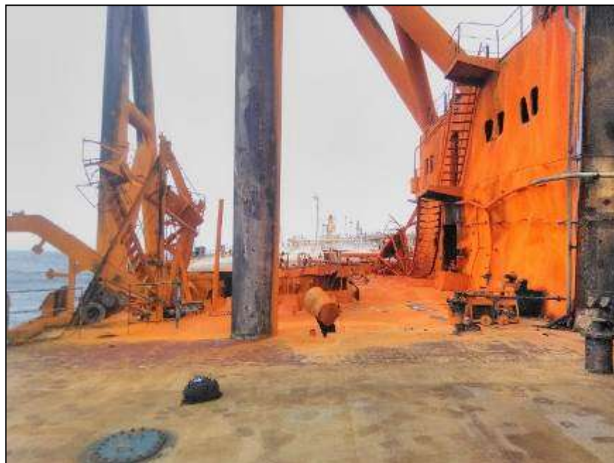
Aft of D/O tank no. 2 deck and in way of aft WB tank appears intact
