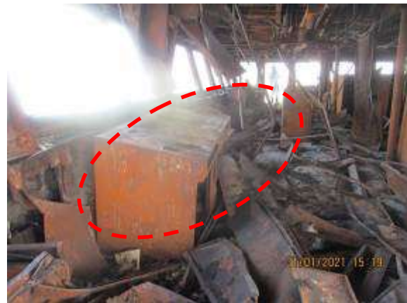
View from Port to STBD side Maneuvering console with burnt out control and engine telegraph
